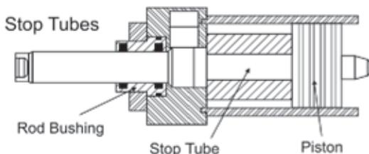
Stop tubes are located between the piston and the rod shoulder on the head end of the cylinder. Bearing loading is reduced by separating the piston and the rod bushing. Bearing wear and tendency to buckle is reduced.
